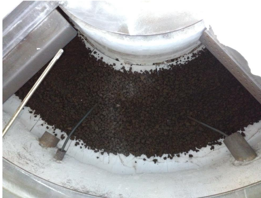
Microwave calcination testing in progress
