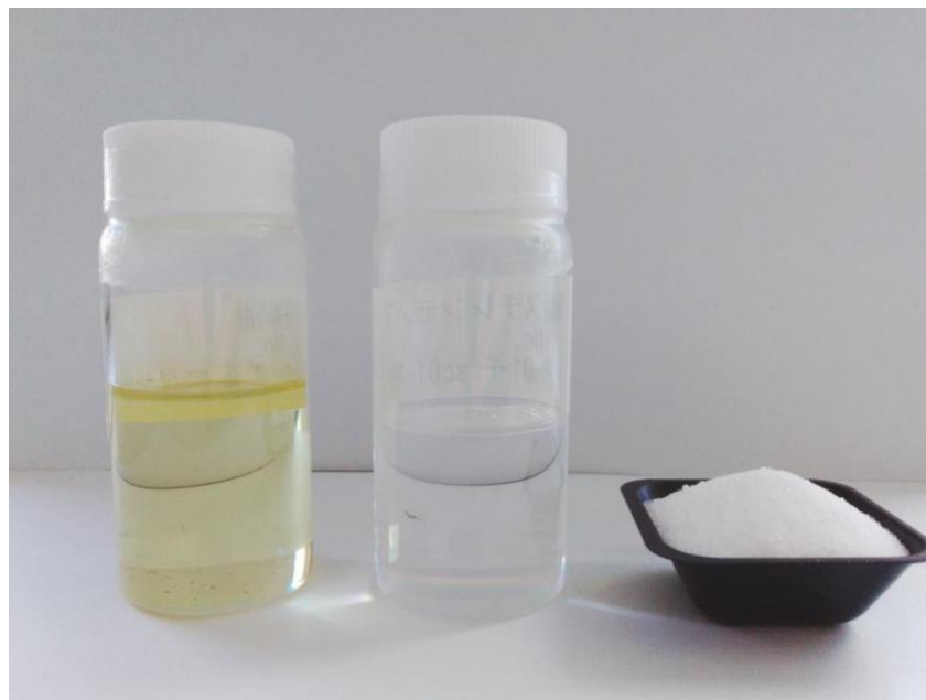
Figure 3 Polystyrene chemically recycled using a small pilot unit (left: decomposed oil / middle: recovered styrene monomer / right: recycled polystyrene)
